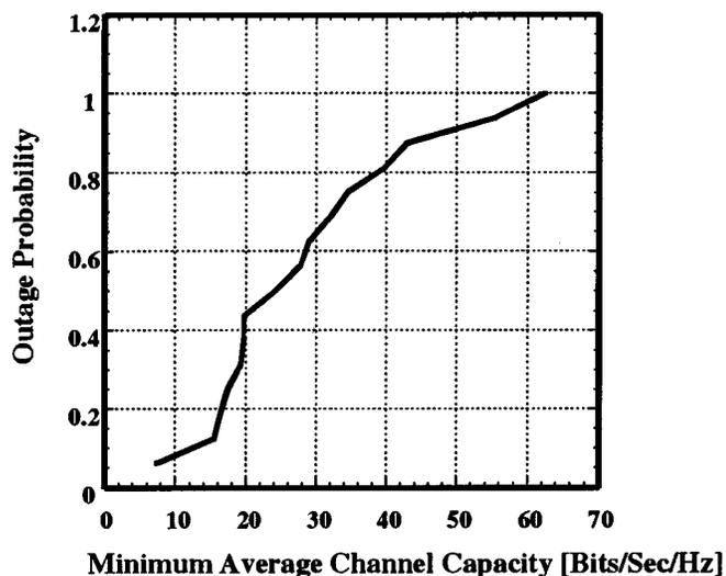
Fig. 18. Cumulative distribution of BLAST capacity for 16 locations. Transmitter power per user = 20 dBm, 10 m remote height.
