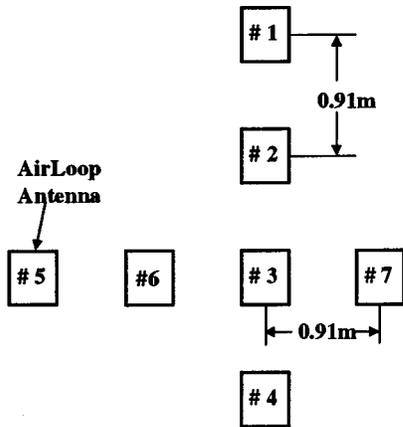
Fig. 2. Front view of asymmetric cross arrangement of the receiving antennas.
