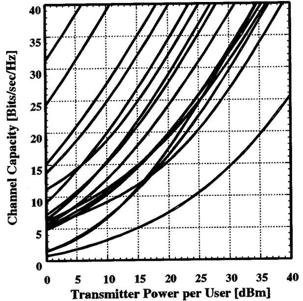
Fig. 16. Average BLAST capacity,  $C_B$ , of the measured sites versus subscriber power.
