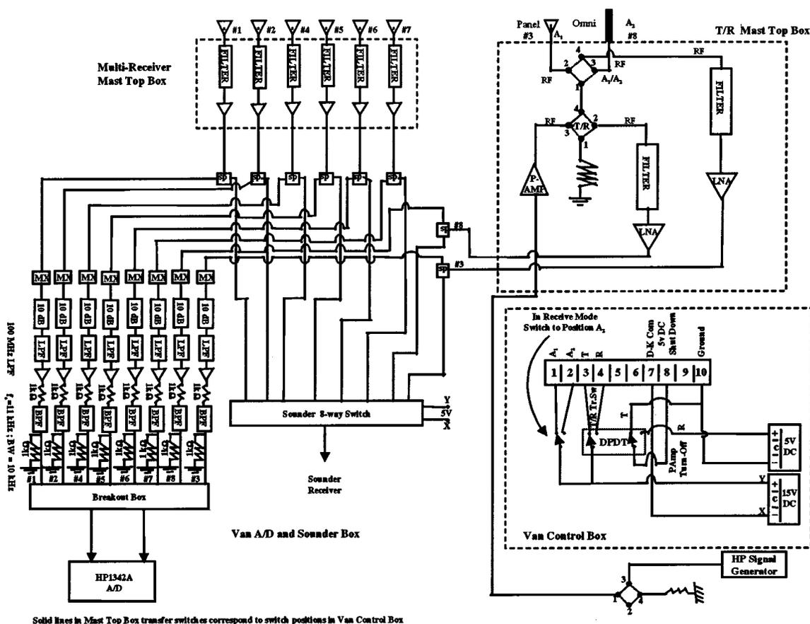
Fig. 4. Schematic diagram of the remote station.
