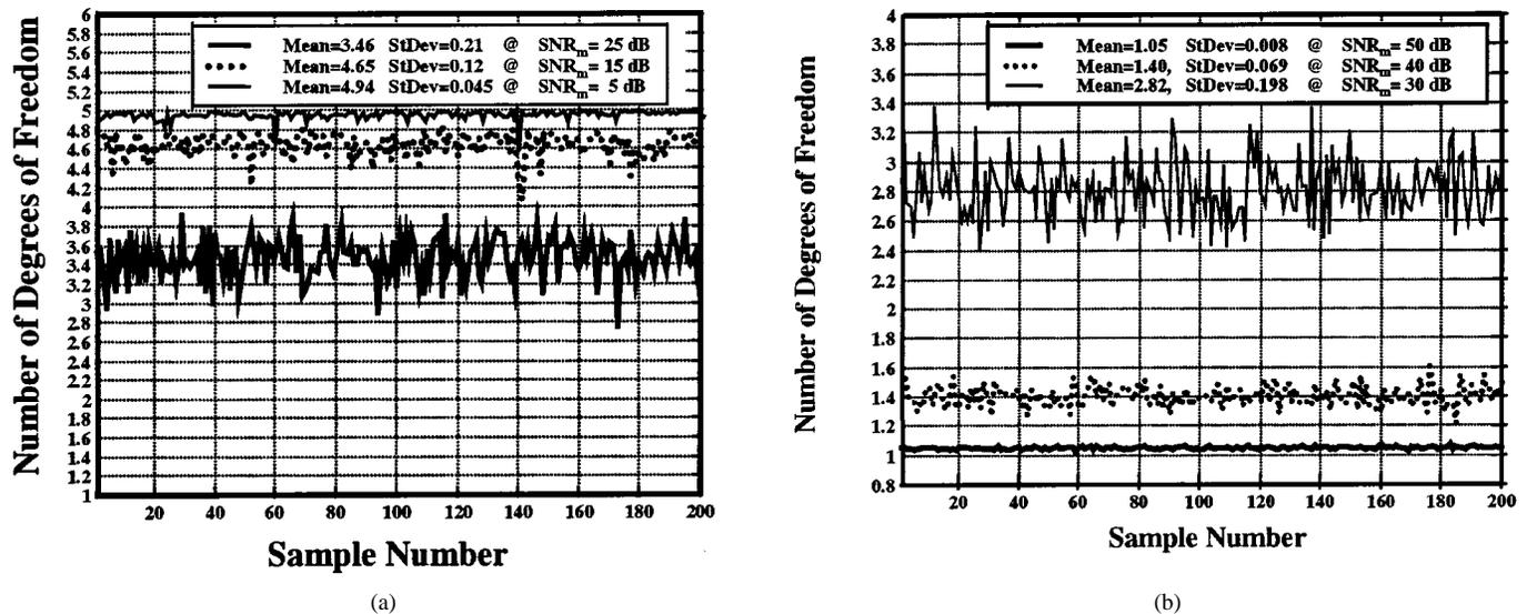
Fig. 5. Number of degrees of freedom ( $D_F$ ) of a  $5 \times 7$  random dyadic keyhole versus sample number. (a)  $\text{SNR}_m = 5\text{--}25$  dB. (b)  $\text{SNR}_m = 30\text{--}50$  dB.
