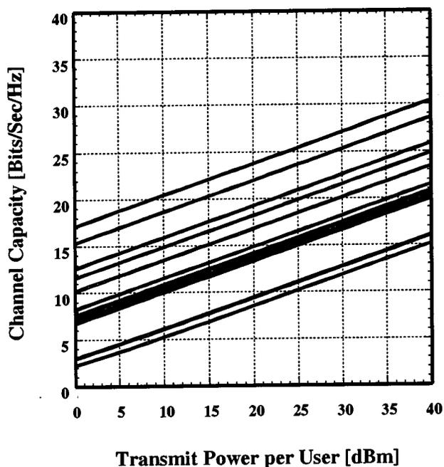
Fig. 17. Extrapolated capacity for focused directive beam (keyholes) in the measured sites versus subscriber power.
