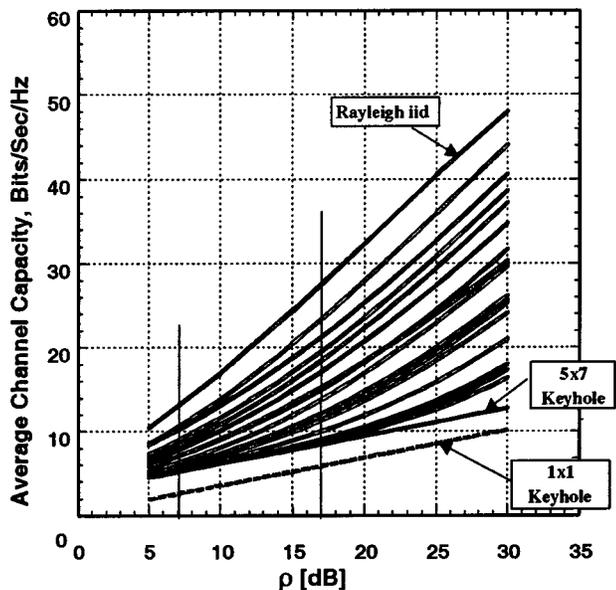
Fig. 13. Average channel capacity,  $C_B$ , versus  $\rho$ . Derived from measurements at 16 locations. Remote subscriber height 10 m.
