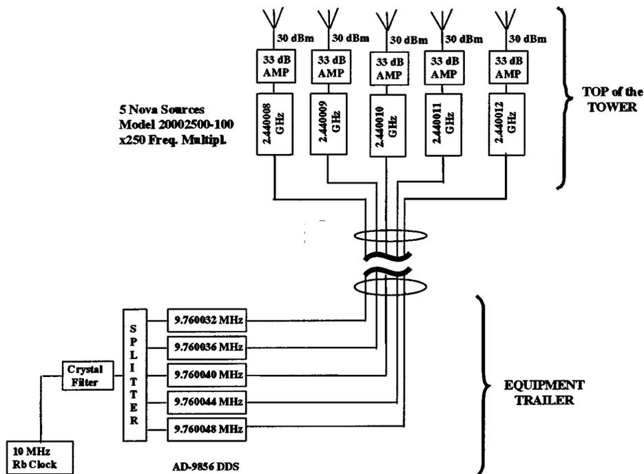
Fig. 3. Schematic diagram of the base station transmitter.
