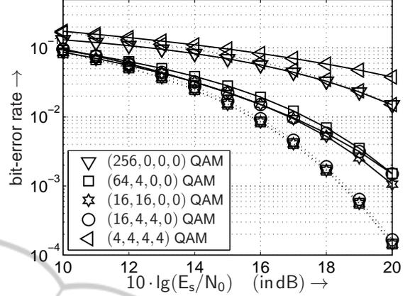
Figure 6: BER with optimal PA (dotted line) and without PA (solid line) when using the transmission modes introduced in Tab. 2 and transmitting 8 bit/s/Hz over channel CM-1.
