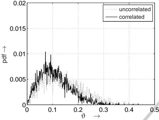
Figure 3: PDF (probability density function) of the ratio  $\vartheta$  between the smallest and the largest singular value for weakly correlated (solid line) as well as uncorrelated (dotted line) frequency non-selective  $(4 \times 4)$  MIMO channel.
