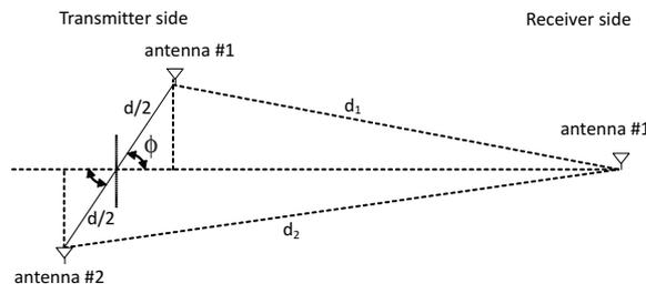
Figure 2: Antennas' physical disposition: two transmit and one receive antennas.
