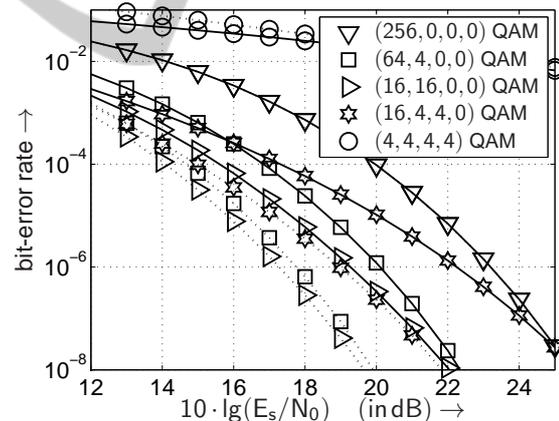
Figure 16: BER with equal-SNR PA (dotted line) and without PA (solid line) when using the transmission modes introduced in Tab. 2 and transmitting 8 bit/s/Hz over frequency non-selective ( $4 \times 4$ ) MIMO channels under weak antenna correlation.
