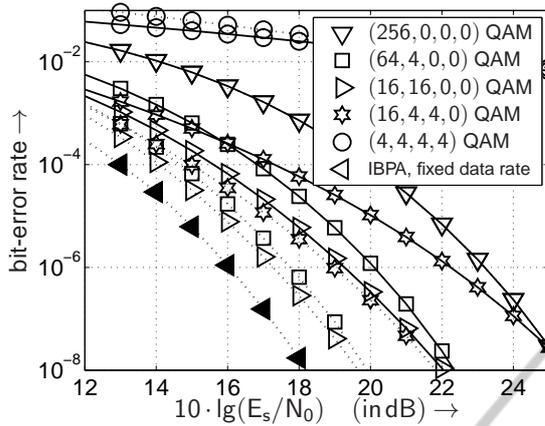
Figure 17: BER with equal-SNR PA (dotted line) and without PA (solid line) when using the transmission modes introduced in Tab. 2 and transmitting 8 bit/s/Hz over frequency non-selective ( $4 \times 4$ ) MIMO channels under weak antenna correlation.
