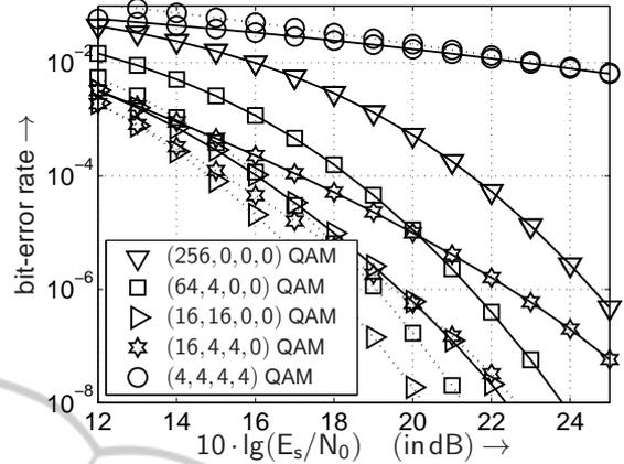
Figure 9: BER with PA (dotted line) and without PA (solid line) when using the transmission modes introduced in Tab. 2 and transmitting 8 bit/s/Hz over non-frequency uncorrelated selective MIMO channels.
