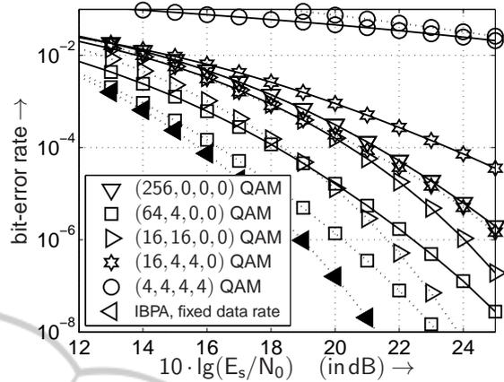
Figure 19: BER with equal-SNR PA (dotted line) and without PA (solid line) when using the transmission modes introduced in Tab. 2 and transmitting 8 bit/s/Hz over frequency non-selective ( $4 \times 4$ ) MIMO channels under strong antenna correlation.
