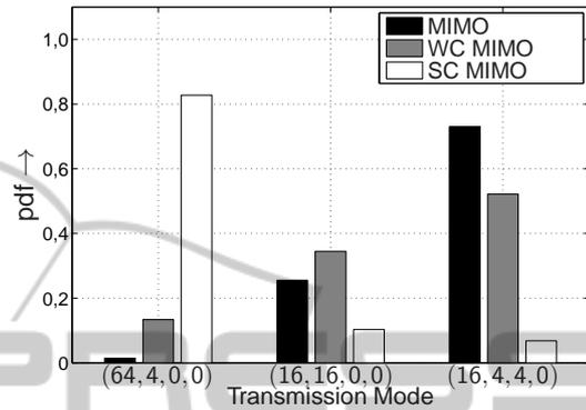
Figure 15: PDF (probability density function) of choosing different transmission modes when using the transmission modes introduced in Tab. 2 and transmitting 8 bit/s/Hz over uncorrelated, weak correlated (WC) and strong correlated (SC) frequency non-selective ( $4 \times 4$ ) MIMO channels.
