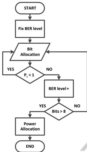
Figure 11: Iterative Bit-and Power Allocation scheme at a fixed data rate.
