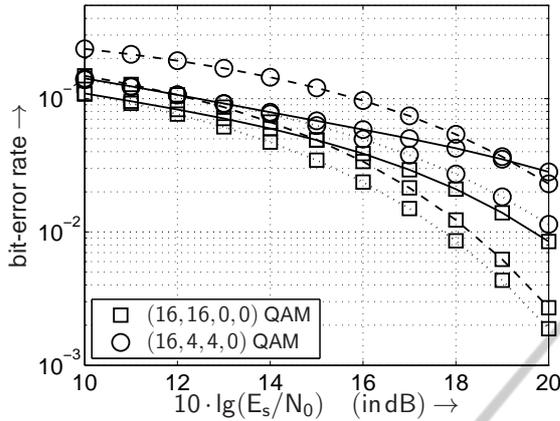
Figure 8: BER with optimal PA (dotted line), equal-SNR PA (dashed line) and without PA (solid line) when using the transmission modes introduced in Tab. 2 and transmitting 8 bit/s/Hz over channel CM-2.
