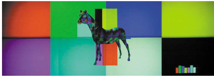
4 Parallel rendering with load balancing. Note the load bars in the lower right.
