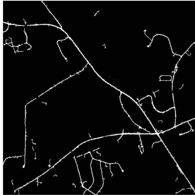
Figure 5. Road features after thresholding. Non-road features have been eliminated.
