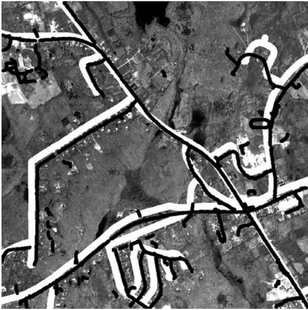
Figure 7. Validation for road extraction. Roads extracted with the methods describe in this paper are displayed in black, and GIS-derived digitized roads are in white and double width. Mis-registration between road layers is due to source material and original projection, yet serve to emphasize differences between the two road layers.
