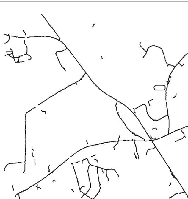
Figure 6. Road centerlines in vector format. Derived from data portrayed in Figure 5.
