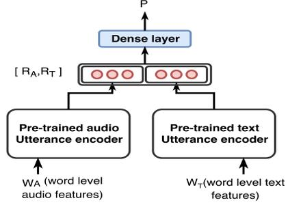
Figure 3: Multimodal system architecture using Comb-LF approach.
