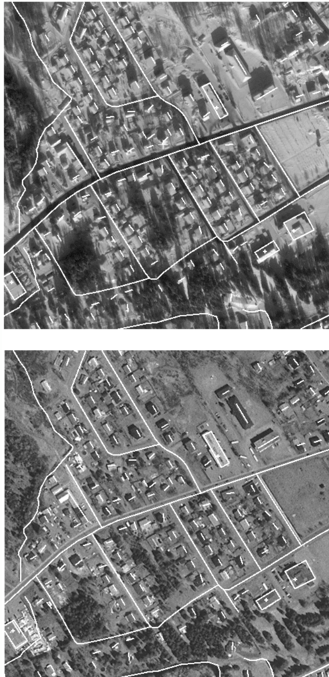
Figure 4. Sub-area of the Beauport_A ortho-image (1-m pixel spacing, 512 pixels 512 lines) at the top, and of the Beauport ortho-photo (1-m pixel spacing, 512 pixels by 512 lines) at the bottom, with 1:25,000 3-m accurate vector lines overlaid.
