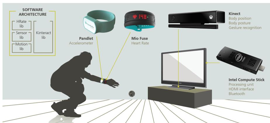
Figure 1: iBoccia architecture.
