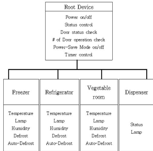
Fig. 8: Function Block of Refrigerator Emulator
