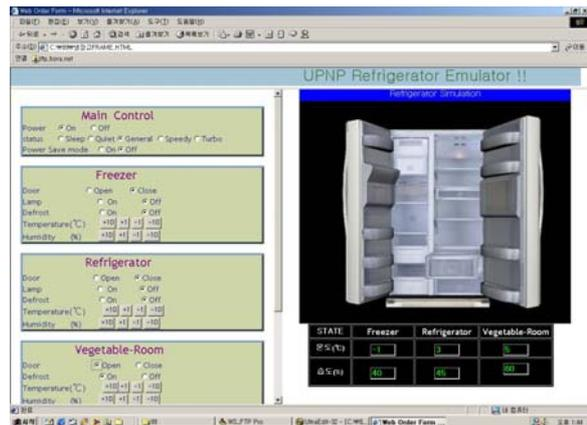
Fig. 9: Display of Refrigerator Emulator
