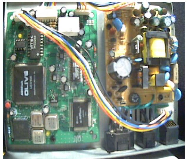
Fig. 6: Ethernet-based High Rate PLC Module
