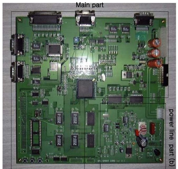
Fig. 5: Prototype of Low Rate PLC Module
