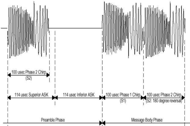
(b) Signal Pattern using the PRK method
