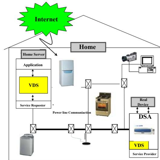
Fig.1 Structure of Home Network System based on PLC
