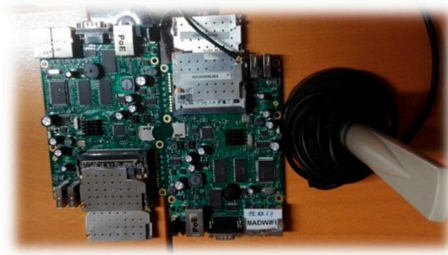
**Figure 4.** Two RB433 UAH MikroTik device, with two Ubiquiti XtremeRange2 and an Ubiquiti XtremeRange5 cards and the corresponding antenna.
