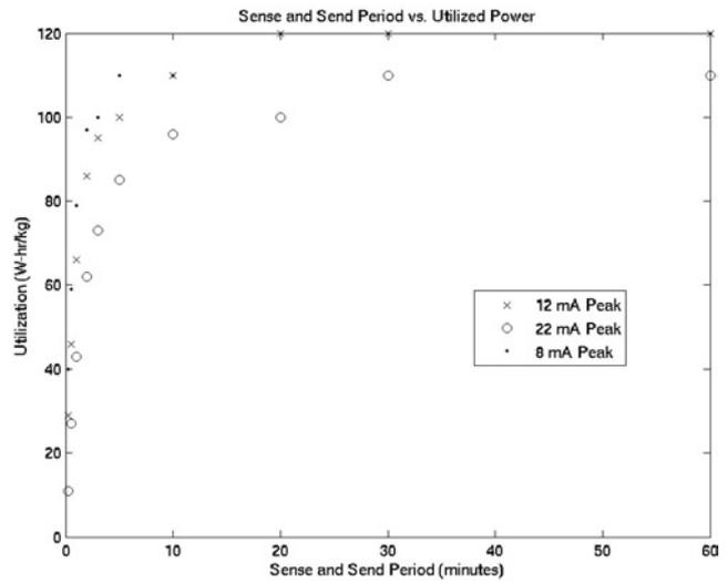
Fig. 4 Battery utilisation for various radios
