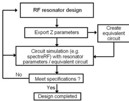
**Fig. 11** Design flow for RF MEMS/CMOS co-design
