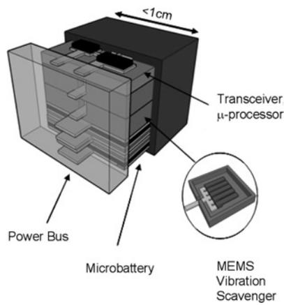
**Fig. 1** Conceptual drawing of  $1 \text{ cm}^3$  sensor node
