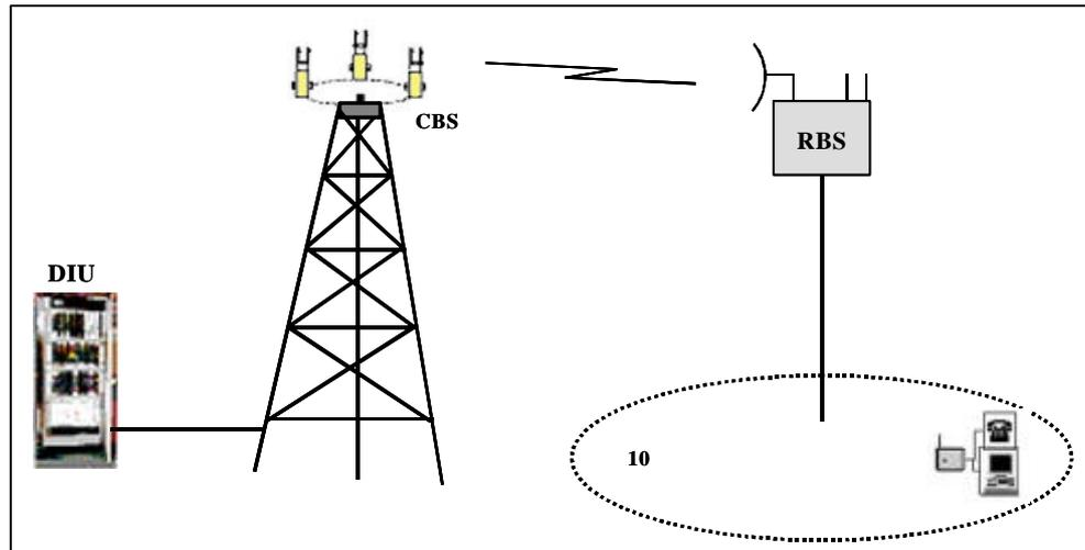
**Fig 5: WS-IP connected to DIU using a two-hop radio link through a Relay Base Station**
