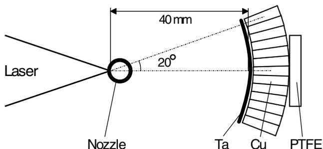
FIG. 1. Schematic drawing of the target setup.
