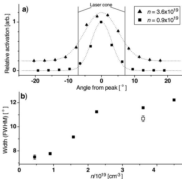
FIG. 2. (a) Normalized angular distributions measured with  $^{62}\text{Cu}$  activation for a low (squares) and a high plasma density ( $\text{cm}^{-3}$ ), offset for clarity. The lines indicate a Gaussian fit to data.  $0^\circ$  is approximately the direction of the laser beam. (b) Width (FWHM) of the electron beam as a function of plasma density. Energy on target was 25–45 J, except a low-energy shot (open square) that was 10 J.
