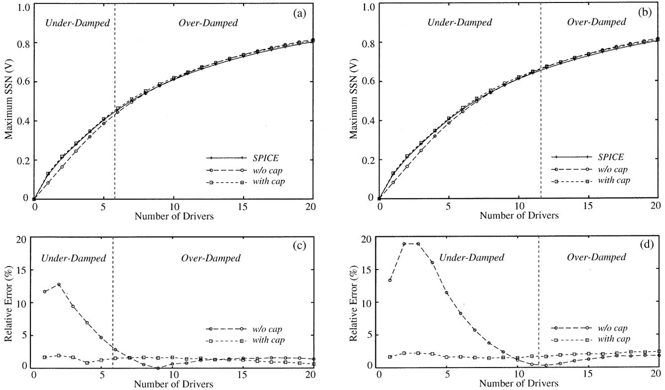
Fig. 6. Comparisons of simulated and calculated maximum SSN voltages. (a)  $L = 5.0$  nH,  $C = 1.0$  pF and  $t_r = 0.50$  ns. (b)  $L = 2.5$  nH,  $C = 2.0$  pF and  $t_r = 0.25$  ns. (c) Relative error of (a). (d) Relative error of (b).
