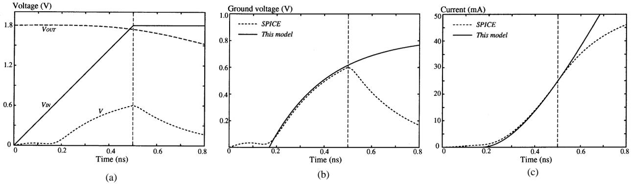
Fig. 3. Comparison of SPICE simulation and model results. (a) Simulated waveforms of ground node and I/O nodes. (b) Simulated and calculated simultaneous switching noise voltage. (c) Simulated and calculated current through the inductor.
