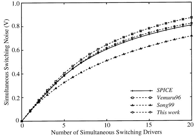
Fig. 4. Comparison with SPICE simulation and with previous works.
