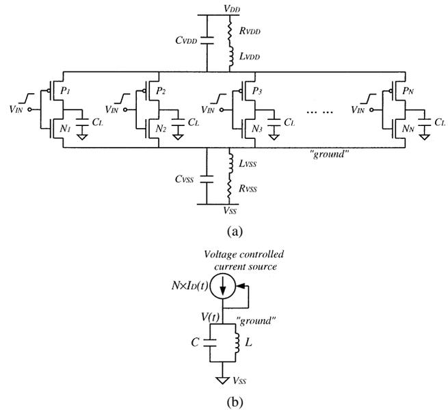
Fig. 1. (a) Equivalent circuit for simultaneous switching noise modeling. (b) Simplified circuit for ground bounce modeling.
