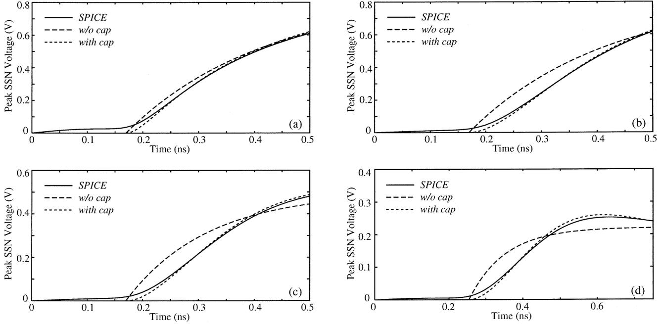
Fig. 5. Comparisons of simulated and calculated SSN waveforms. (a) Case 1: over damped,  $L = 5.0$  nH,  $C = 1.0$  nF,  $t_r = 0.50$  ns,  $N = 10$ . (b) Case 2: critically damped,  $L = 5.0$  nH,  $C = 3.0$  nF,  $t_r = 0.50$  ns,  $N = 10$ . (c) Case 3a: under damped,  $L = 5.0$  nH,  $C = 2.0$  nF,  $t_r = 0.50$  ns,  $N = 6$ . (d) Case 3b: under damped,  $L = 5.0$  nH,  $C = 2.0$  nF,  $t_r = 0.75$  ns,  $N = 4$ .
