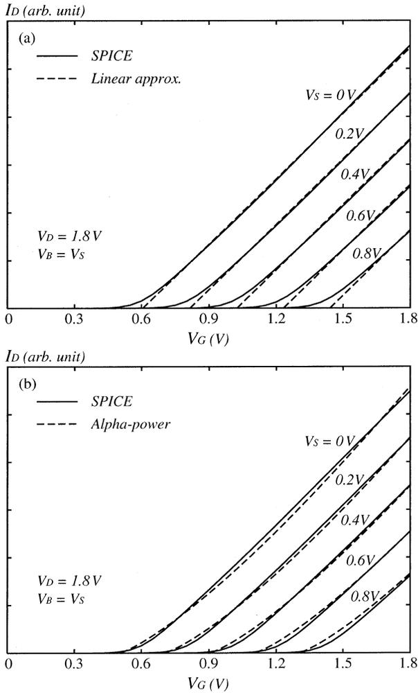
Fig. 2. MOSFET  $I$ - $V$  characteristic modeling. (a) Linear approximation. (b)  $\alpha$ -power law model.
