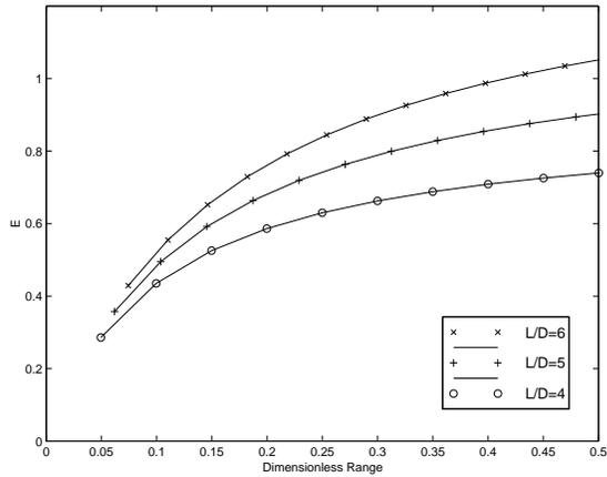
Figure 10: Range/Mass Efficiency Number (E) of PHC Trajectories
