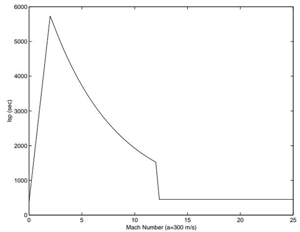
Figure 8:  $I_{sp}$  vs. Mach Number for RBCC Engine
