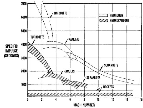
Figure 7: Variation of  $I_{sp}$  with Mach Number for Various Engine Technologies
