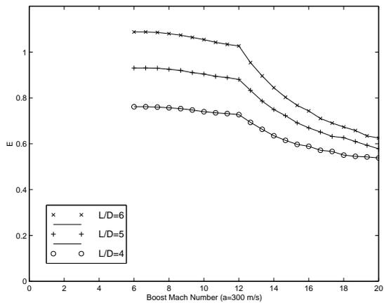
Figure 11: Range/Mass Efficiency Number (E) of PHC Trajectory vs. Boost Velocity
