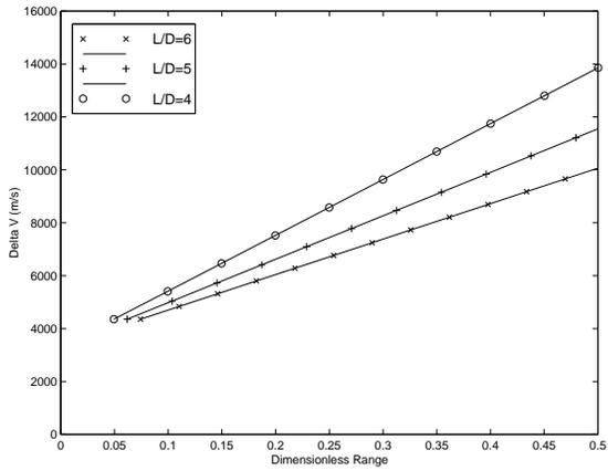
Figure 3:  $\Delta V_{Total}$  vs.  $\phi_{Total}$  of a PHC Trajectory
