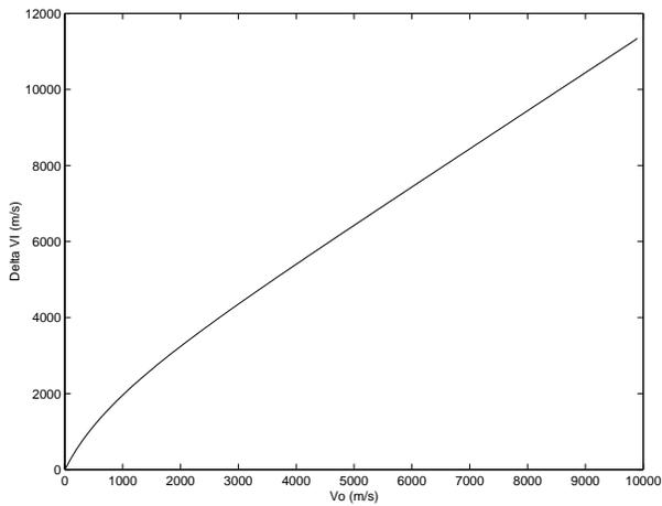
Figure 4:  $\Delta V_I$  vs.  $V_o$  for  $V_i=0$
