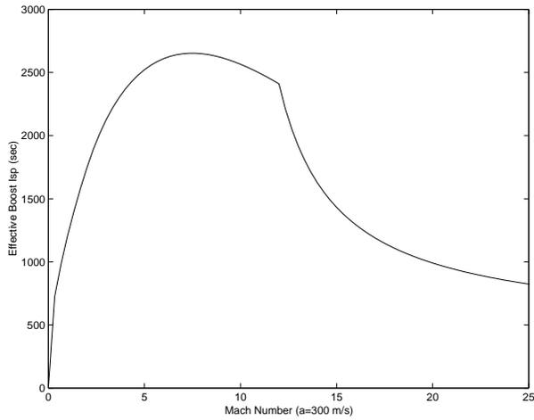
Figure 9:  $I_{sp}^{e-Boost}$  vs. Boost Mach Number for RBCC Engine Boosting from Takeoff
