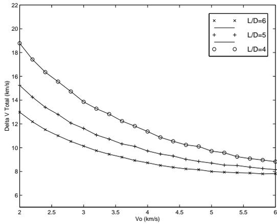
Figure 5:  $\Delta V_{Total}$  vs.  $V_o$  for 20,000 km Range PHC Trajectory
