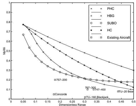
Figure 13: Comparison of Payload Carrying Capability of Vehicles Flying Various Trajectory Forms
