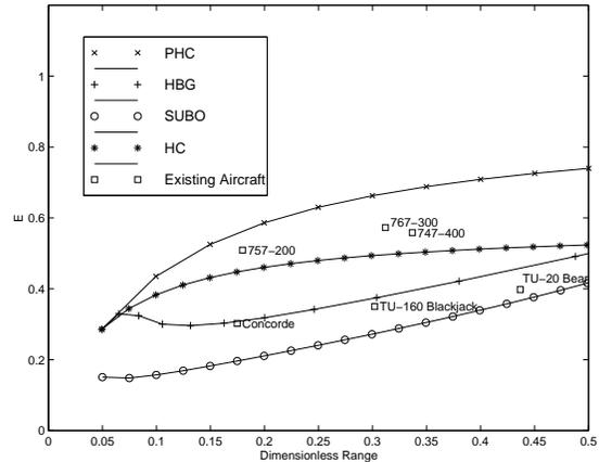
Figure 12: Range/Mass Efficiency Number (E) vs. Range of Various Trajectory Forms
