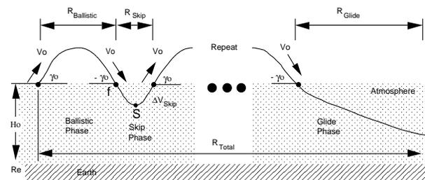
Figure 2: Parameters of a Periodic Hypersonic Cruise Trajectory
