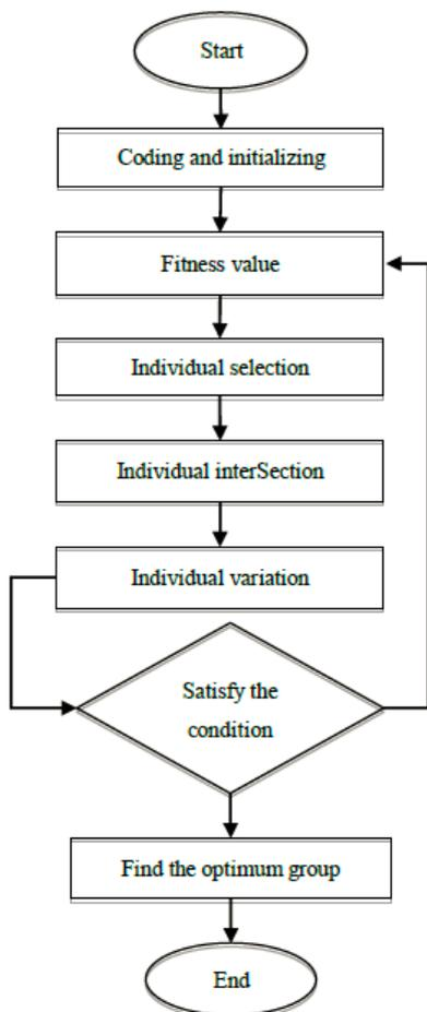
Figure 2. Flow chart for genetic algorithm
