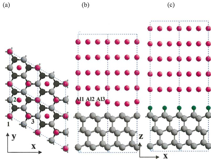
FIG. 1. (Color) Relaxed interfaces. (a) and (b) Projection of Al/C-1 $\times$ 1 ( $a=b=5.027$  Å,  $c=34.815$  Å) along  $z$  and  $y$ , respectively. (c) Projection of Al/C-1 $\times$ 1:H ( $a=b=5.018$  Å,  $c=40.075$  Å) along  $y$ . Atom colors: Al, pink; C, gray (first layer) and black (second layer); H, green.
