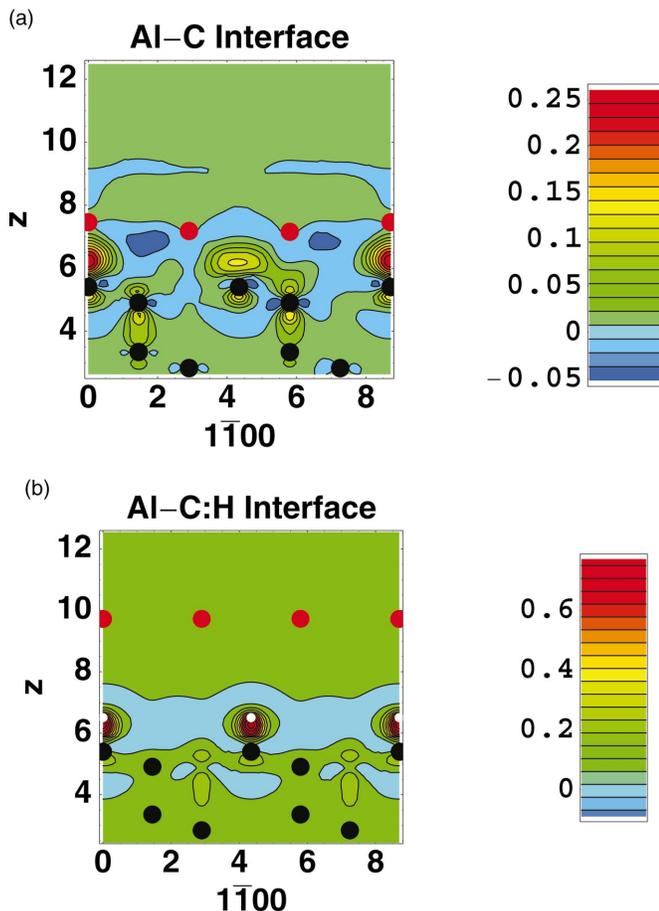
FIG. 2. (Color) Charge density differences ( $\rho/\text{Å}^3$ ) along relaxed interfaces. (a) Al/C-1 $\times$ 1. (b) Al/C-1 $\times$ 1:H, with red, black, and white representing atomic positions of Al, C, and H, respectively.
