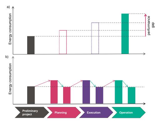
Fig. 1: Qualitative visualization of the performance gap that occurs throughout a project's phases (a) and the closing of the gap by pairing the project with a digital twin (b).
