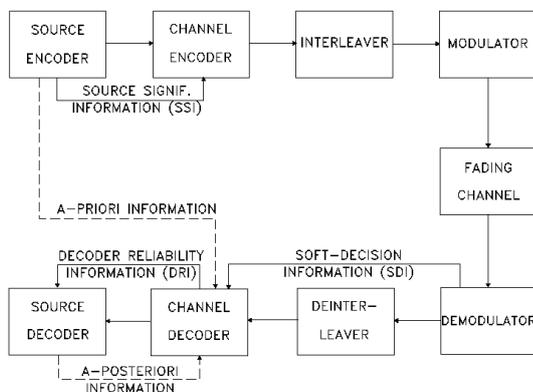
Figure 1: Intelligent transceiver schematic.
