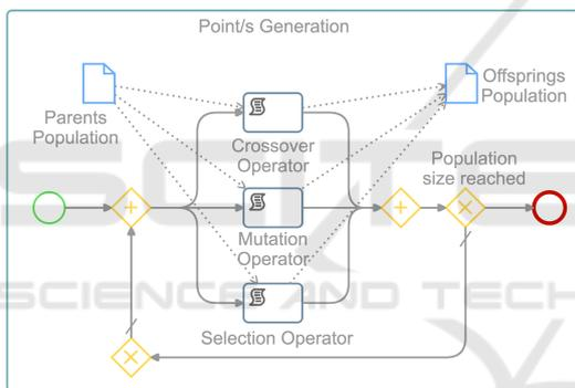
Figure 5: A possible specialization of the sub-process responsible for the generation of new configurations. In this example we show a Genetic Algorithm with parallel operators.
