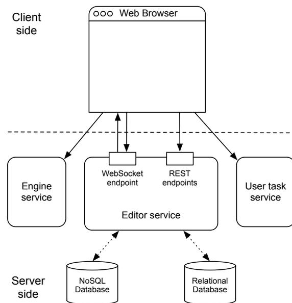
Figure 1: Web application architecture. Straight lines represent communication over HTTP, while dotted lines represent database read/write operations.
