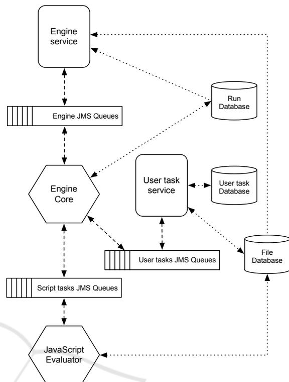
Figure 2: BPMN engine architecture. Dashed lines represent send/receive operations to/from JMS queues, while dotted lines represent database read/write operations.
