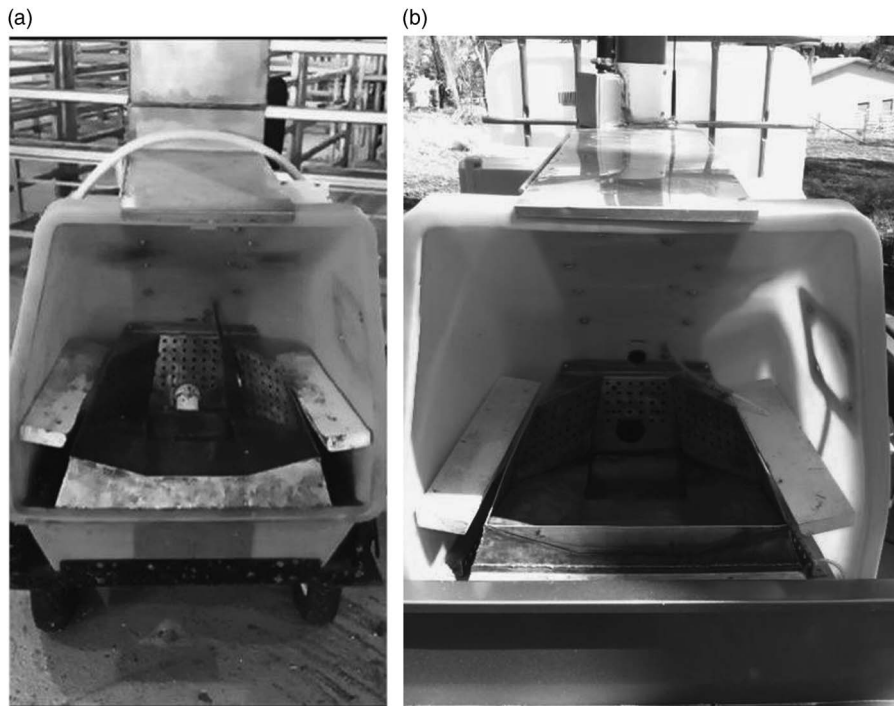
Figure 1 GreenFeed Emission Monitoring (GEM) units showing shroud where cattle enter to receive a pelleted supplement (GEM supplement; a) or water (GEM water; b) based on animal RFID identification.
