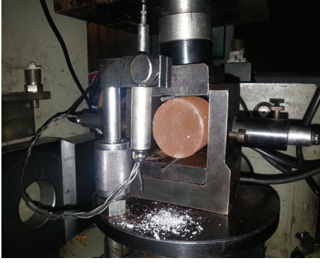
FIGURE 2: Photo of salt rock specimens on loading.
