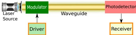
Figure 1. An optical communication system
