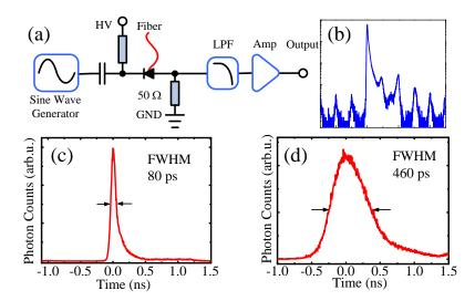
Fig. 2. (color online) (a) Schematic of the InGaAs/InP APD SPD. LPF: low-pass filter; HV: bias voltage; Amp: RF amplifier (gain: 13 dB, bandwidth: 3 GHz). (b) Avalanche trace of the APD output. Timing jitter of the single-photon with (c) and without (d) synchronization to the laser pulse.
