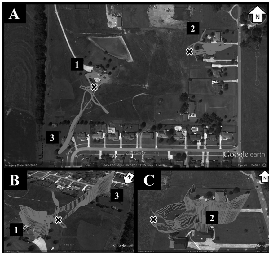
Figure 2. Graphic depicting telemetry data recorded from UAS reconnaissance flights (© Google Earth): (A) Nadir view of flight plan for observing Structures 1 to 3. Isometric views of flight plans for (B) Structures 1 and 3, and (C) Structure 2. Telemetry data including latitude, longitude and altitude above was collected onboard the UAS during flight. Structures 1 and 2 were assessed by multiple UAS passes originating at the locations marked with a black “x.”
