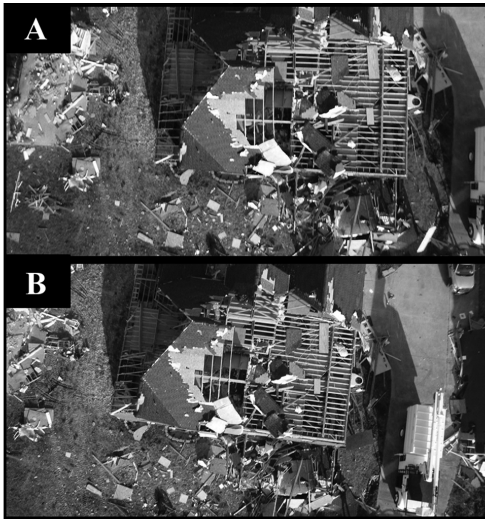
Figure 9. Two overlapping nadir images of Structure 2, potentially useable for stereo-photogrammetric analysis to estimate three-dimensional coordinates of different points on the building.
