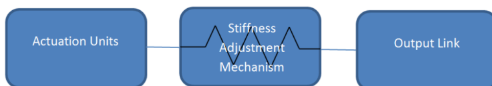
Figure 1. The concept of a stiffness adjustment mechanism and transmitted energy within the system.
