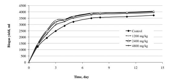
Fig.3. Biogas yield during 14 days of anaerobic digestion at various Ni(II) concentrations
