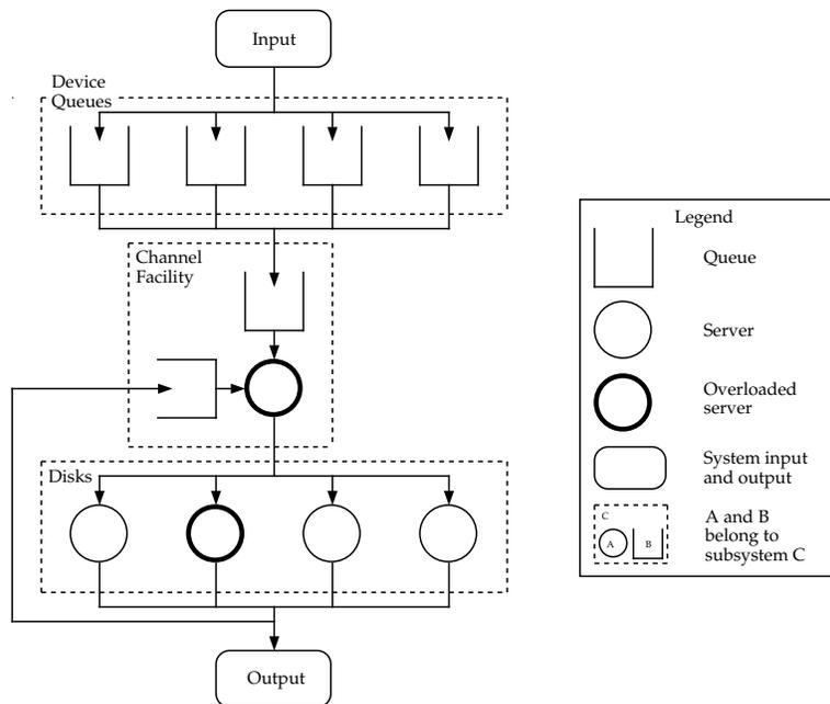
Figure 1: The disk subsystem of a computer
