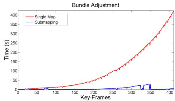
Figure 5: Bundle adjustment computation time (offline) with and without partitioning.
