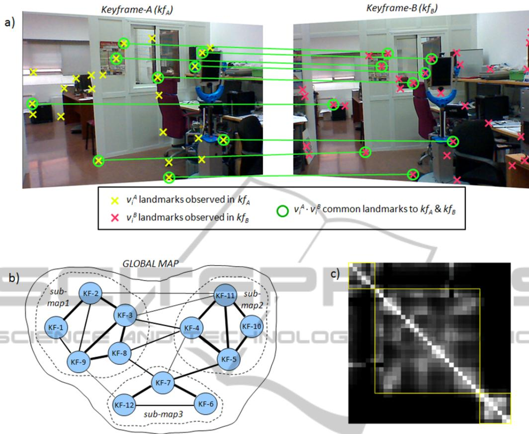
Figure 1: a) Common observations between two keyframes. This is used to calculate the *Sensed Space Overlap* (SSO) (see equation 5). b) Graph-representation of the map where each node represents a keyframe and the arcs are weighed with the SSO calculated between keyframes (thicker arcs mean higher SSO). c) Example of SSO matrix, in which the brightness of the element  $ij$  represents the SSO between the keyframes  $i$  and  $j$ .
