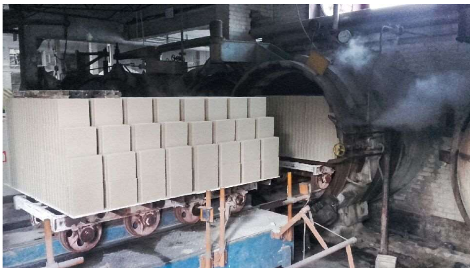
Fig. 2. Specimens subjected to autoclaving process in industrial conditions.
