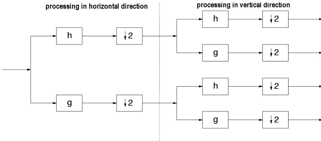
Figure 1. One stage filterbank implementation of a two-dimensional discrete wavelet decomposition.
