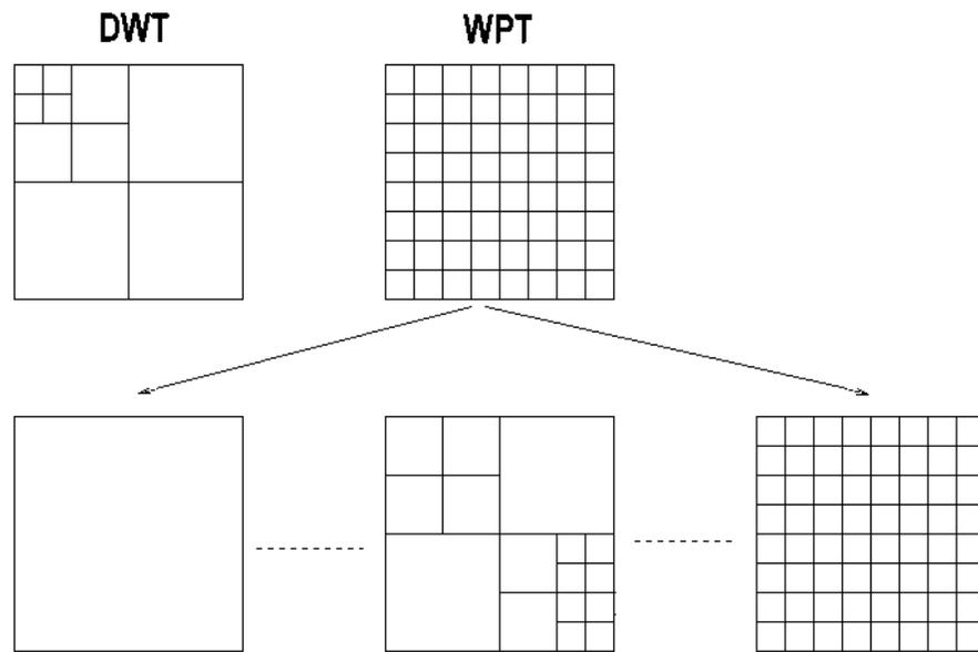
Figure 4. Decomposition bases offered by DWT and WPT.
