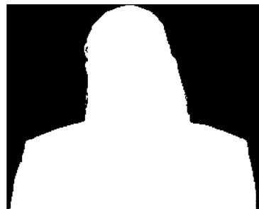
Fig. 5. Shape of the first I-VOP of the AKIYO video object.
