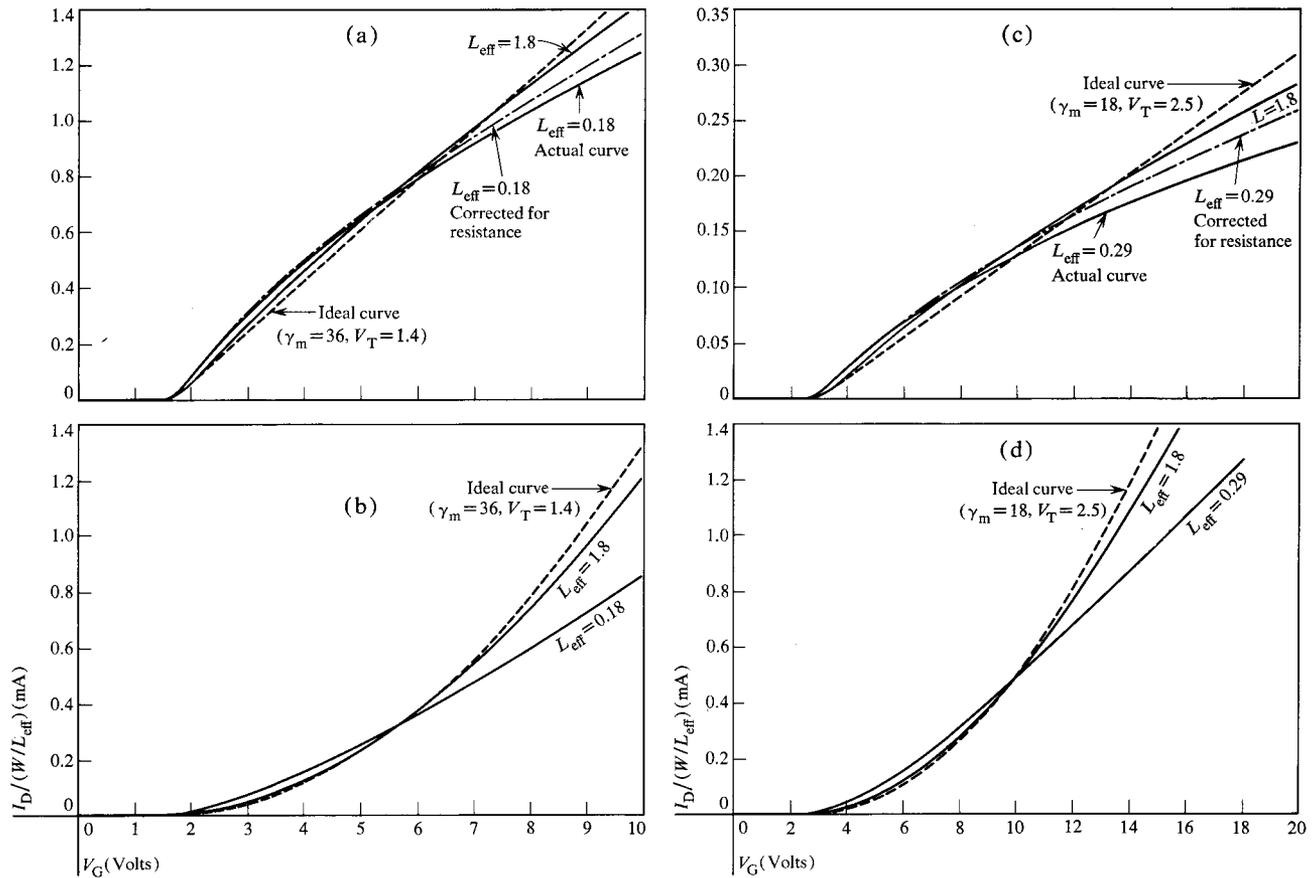
Figure 16 Normalized transfer characteristics above and below pinchoff for long and short channel lengths. (a)  $500\text{\AA}$ ,  $V_D = 0.5\text{V}$ ; (b)  $500\text{\AA}$ ,  $V_D = 10\text{V}$ ; (c)  $1000\text{\AA}$ ,  $V_D = 1.0\text{V}$ ;  $1000\text{\AA}$ ,  $V_D = 16\text{V}$ .
