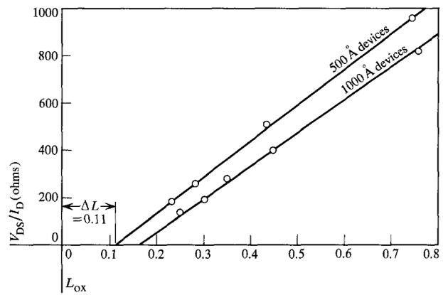
Figure 15 Experimental values from Fig. 14, plotted to allow determination of  $\Delta L$ .
