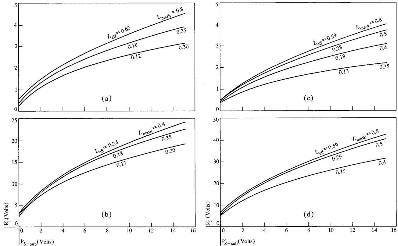
Figure 17 Threshold voltage vs source-to-substrate voltage for various channel lengths. (a)  $500 \text{ \AA}$ ,  $V_D = 6V$ ; (b)  $6000 \text{ \AA}$ ,  $V_D = 6V$ ; (c)  $10000 \text{ \AA}$ ,  $V_D = 12V$ ; (d)  $10,000 \text{ \AA}$ ,  $V_D = 12V$ .
