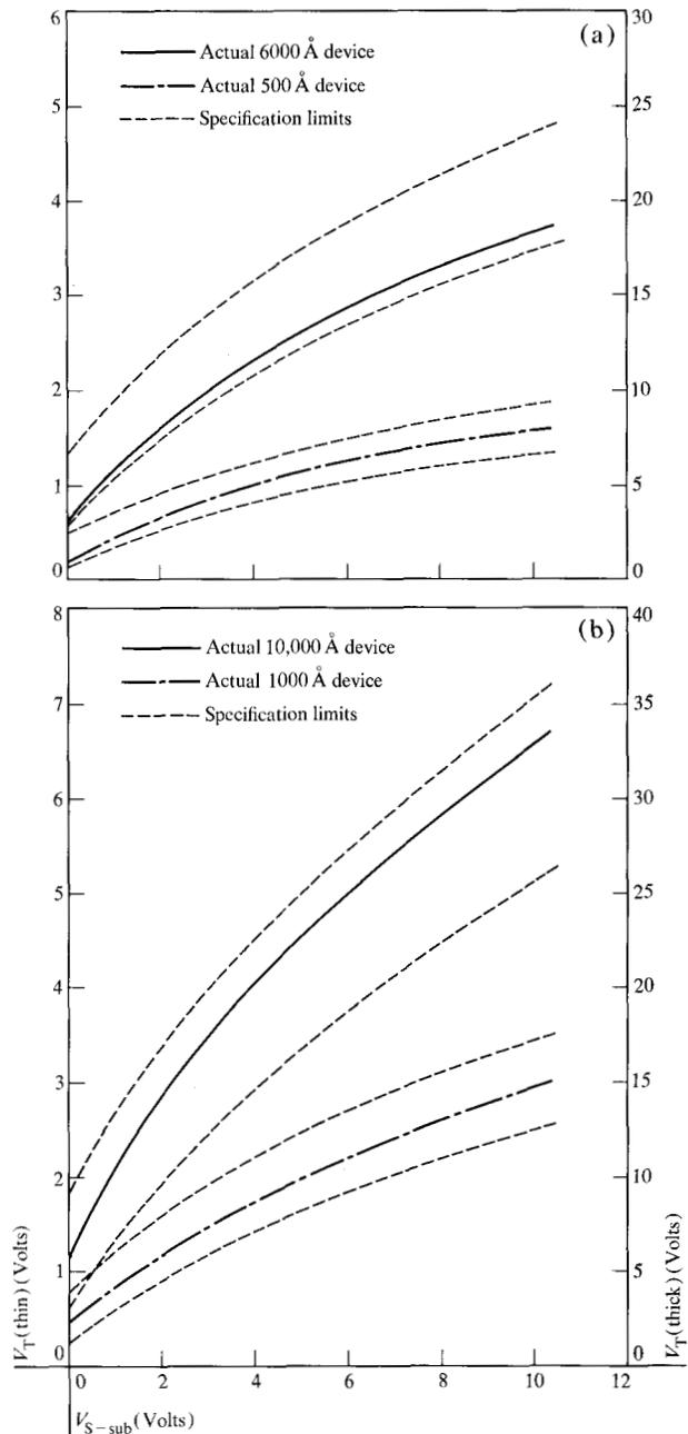
Figure 11 Measured threshold voltage vs source-to-substrate voltage (compared with initial specification limits) for the short-L devices characterized in the preceding figures.
