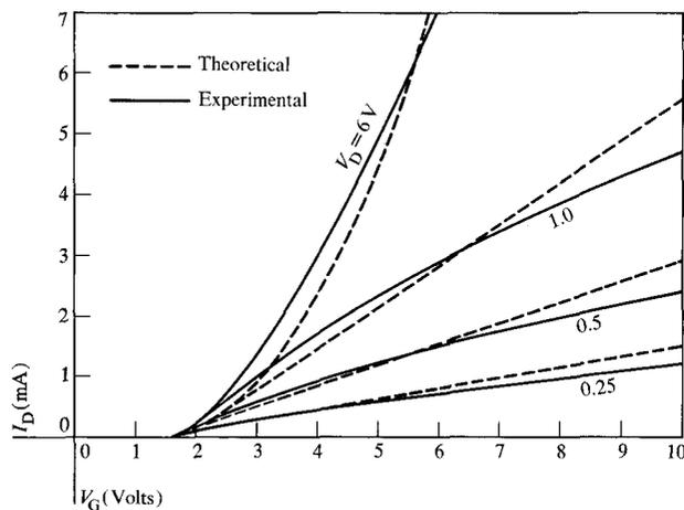
**Figure 3** Transfer characteristics of a 500 Å device compared with theoretical device equations for constant  $\gamma_m$ . ( $W = 4$  mil;  $L_{\text{eff}} = 0.18$  mil.)
