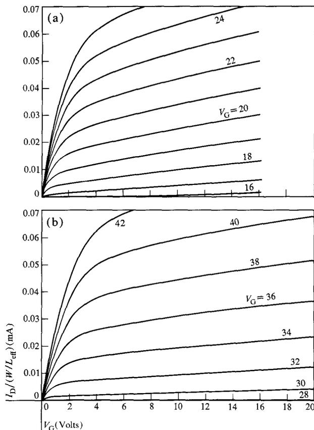
Figure 9 Characteristics of parasitic thick-oxide devices. (a)  $6000\text{\AA}$ ,  $L = 0.35$  mil ( $L_{\text{eff}} = 0.19$  mil,  $R_D W/L_{\text{eff}} = 800\Omega$ ,  $R_S W/L_{\text{eff}} = 8\text{k}\Omega$ ); (b)  $10,000\text{\AA}$ ,  $L = 0.50$  mil ( $L_{\text{eff}} = 0.29$  mil,  $R_D W/L_{\text{eff}} = 350\Omega$ ,  $R_S W/L_{\text{eff}} = 4.1\text{k}\Omega$ ).
