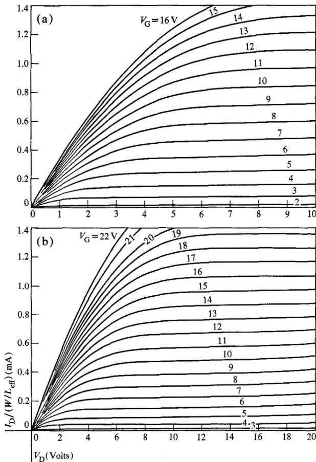
Figure 7 Normalized grounded-source characteristics. (a) 500Å device,  $L = 0.35$  mil,  $L_{\text{eff}} = 0.18$  mil ( $R_D W/L_{\text{eff}} = 110\Omega$ ,  $R_S W/L_{\text{eff}} = 75\Omega$ ); (b) 1000Å device,  $L = 0.5$  mil,  $L_{\text{eff}} = 0.29$  mil ( $R_D W/L_{\text{eff}} = 400\Omega$ ,  $R_S W/L_{\text{eff}} = 60\Omega$ ).
