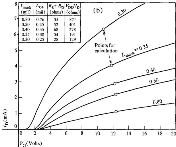
Figure 14 Transfer characteristics for various channel lengths ( $W = 4$  mil). (a) 500Å devices,  $V_D = 0.5V$ ; (b) 1000Å devices,  $V_D = 1.0V$ .
