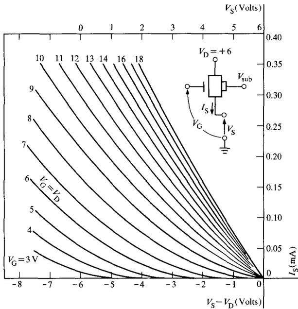
Figure 5 Grounded-drain (load device) characteristics. (500 Å device:  $W/L_{\text{eff}} = 1/4$ .)
