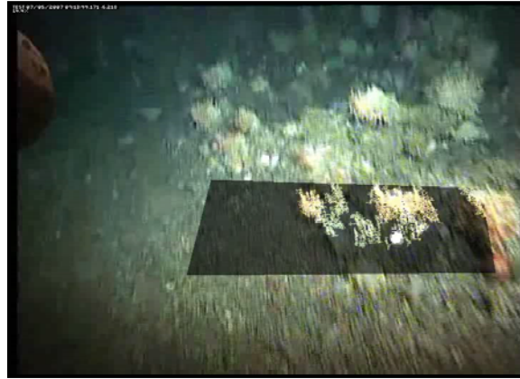
Figure 5. Example of candidate regions detected from motion analysis (stony coral at approximately 1,000 m depth). The ‘footprint’ area of analysis can be specified and is shown here as a grey trapezoid.
