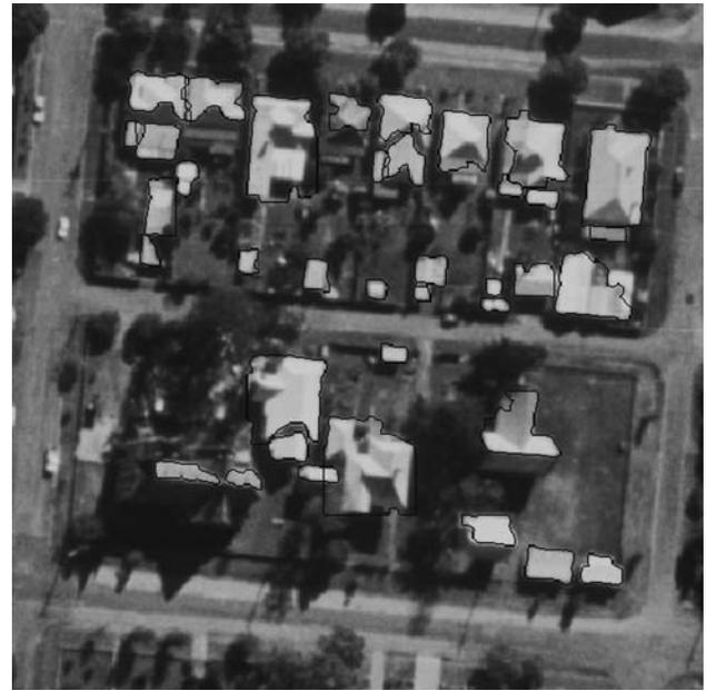
Figure 7. Detected buildings overlaid on the ortho image.
