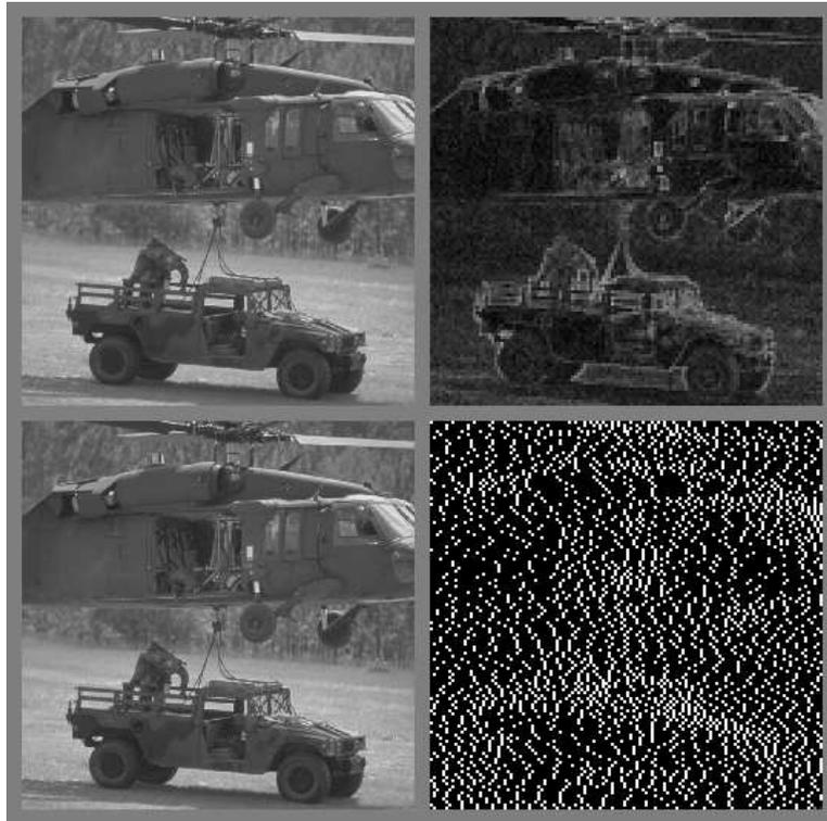
Figure 8: (a) Top left: original  $1024 \times 1024$  grayscale image. (b) Top right: spatial distribution of the number of bytes in each  $8 \times 8$  block after Huffman binary encoding. (c) Bottom left: decompressed JPEG image. (d) Bottom right: spatial distribution of the number of bytes in each  $8 \times 8$  block after output of pipelining realignment algorithm.
