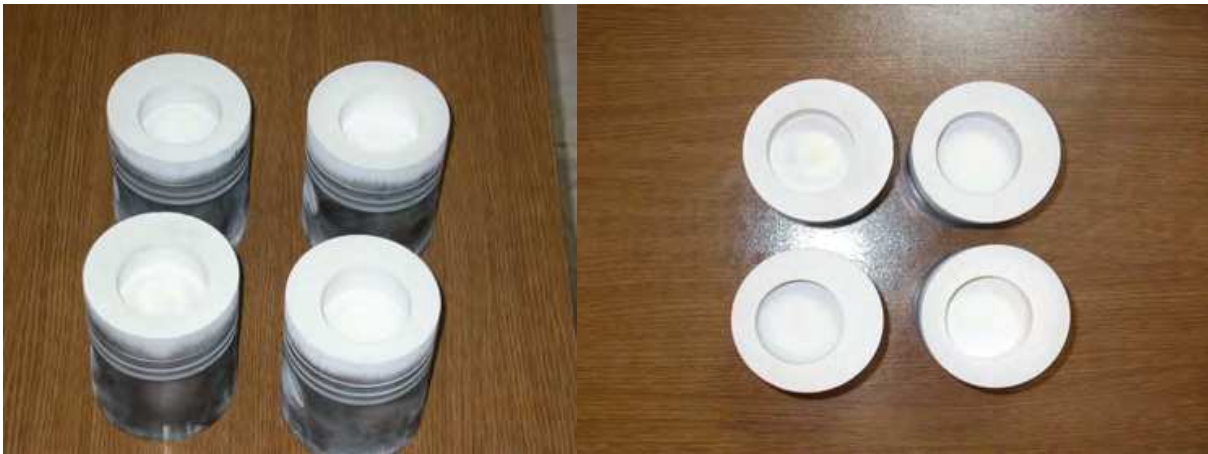
Fig. 10. Ceramic coated piston tops
