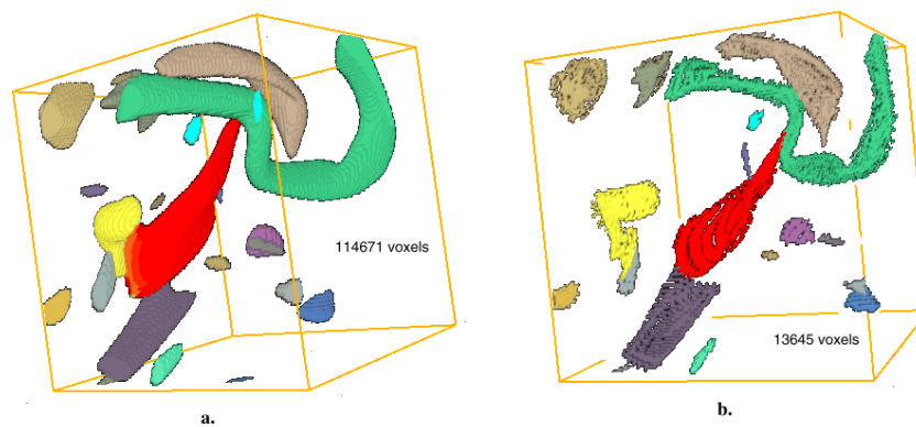
Figure 13: Skeletons for fast Vortex Tracking. (a) Segmented vortex structures.(b) Skeleton of these structures, thinness = 1.0
