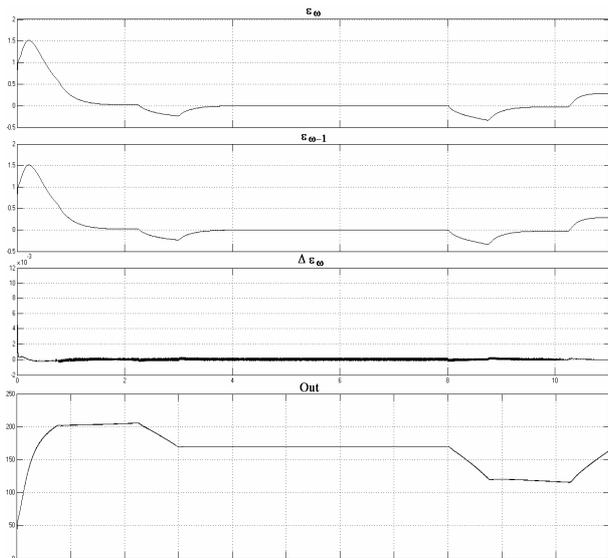
Figures 8: The data training set: the speed error, its variation and the saturated output for the initial speed controller.
