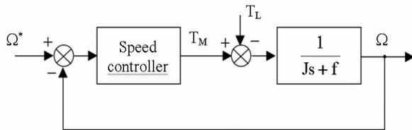
Figures 2: For the speed controller tuning.
