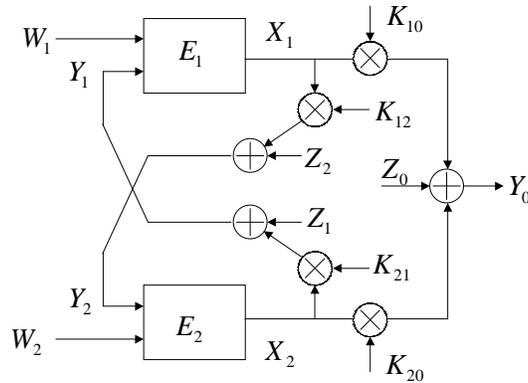
FIGURE 1. Block diagram of a fading Gaussian cooperative channel
