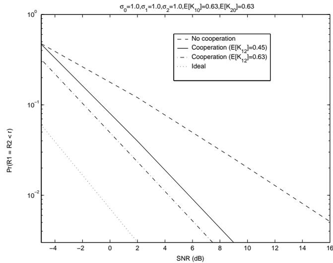
FIGURE 5. Probability of outage versus signal to noise ratio for two-user cooperative system. Both users have similar average quality links towards the destination. The common operating rate is  $r = 0.18$ .
