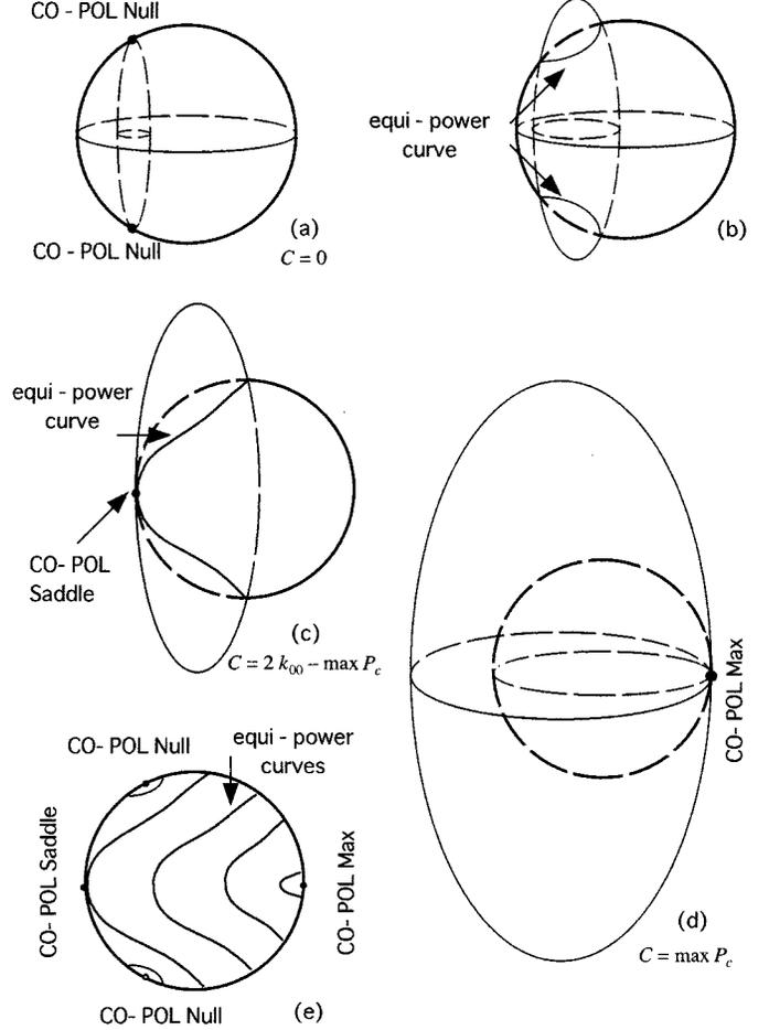
Fig. 2. Equi-power curves and the characteristic polarization states in the co-pol channel.
