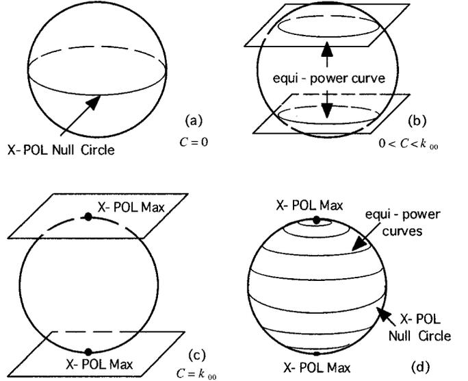
Fig. 6. Equi-power curves in the case of the cross-pol channel when  $\mathbf{G}_c^2(n) = -\mathbf{G}_c^1(n)$ .
