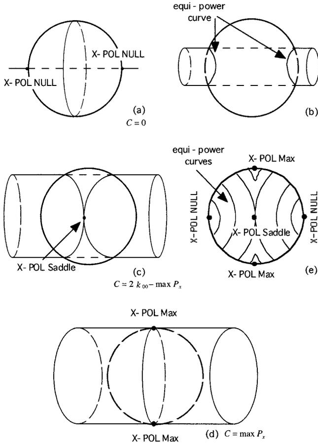
Fig. 3. Equi-power curves and the characteristic polarization states in the cross-pol channel.
