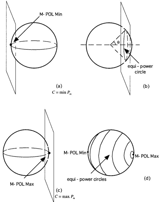
Fig. 4. Characteristic polarization states and the equi-power curves in the matched-pol channel.
