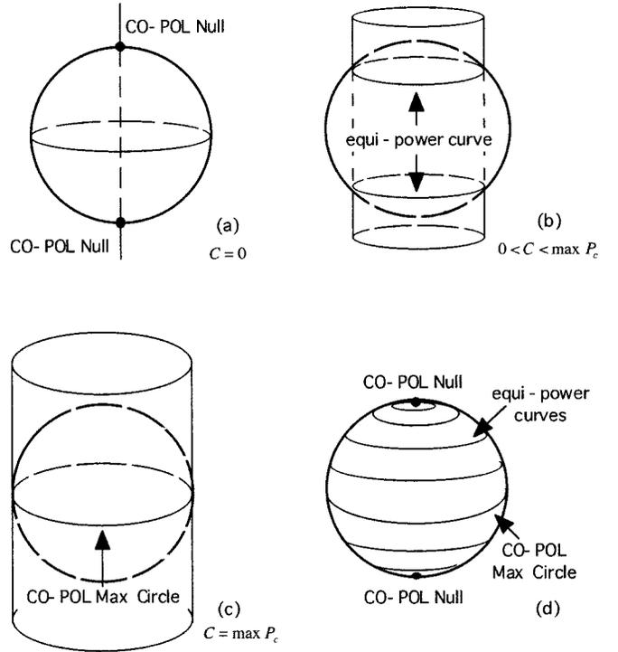
Fig. 5. Equi-power curves in the case of the co-pol channel when  $\mathbf{G}_c^2(n) = -\mathbf{G}_c^1(n)$ .
