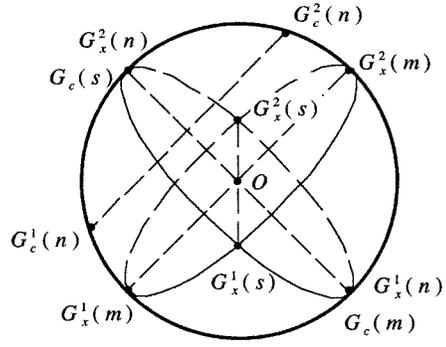
Fig. 1. Characteristic polarization states on the Poincaré sphere.
