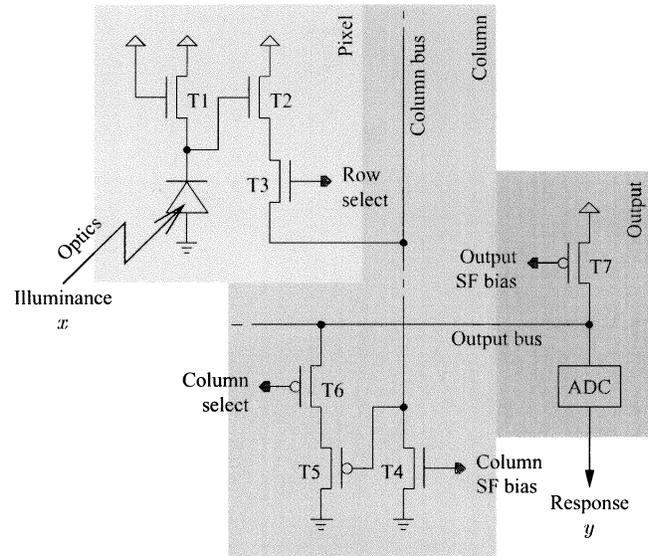
Fig. 1. From an illuminance  $x$  to a digital response  $y$  in one pixel of a logarithmic CMOS image sensor. T2 with T4 and T5 with T7 form an NMOS and PMOS source follower (SF), respectively, when T3 and T6 are turned on.
