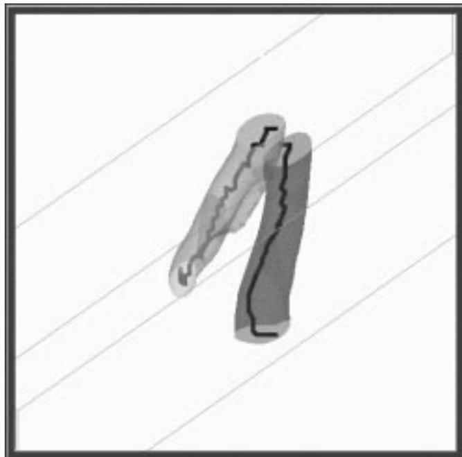
Figure 12: Vortex cores reduced to a skeleton representation.
