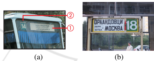
Figure 3: On and inside a tram: (a) Front of a tram displaying route number (in this example route 14), the service identifier, and destination names. The destination name of both ends of the line are shown. Ideally, only the actual direction the vehicle is traveling in should be shown. (b) The inside signboard of a tram where the red arrow shows the ‘direction’ the tram is going.
