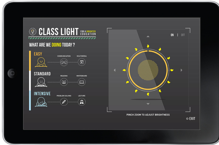
Fig. 5. Dynamic lighting system implemented as a mobile application with three lighting presets.
