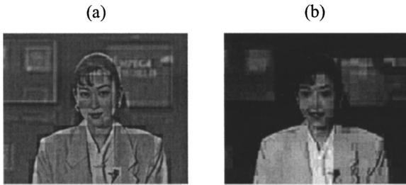
**Fig. 6** Inverse quantization test. (a)  $QP=1$ ,  $dc\_scaler=2$ , (b)  $QP=29$ ,  $dc\_scaler=58$ .
