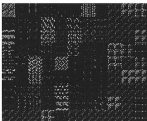
**Fig. 7** Difference picture between the output of the reference decoder and that of the hypothetical decoder for a P frame.
