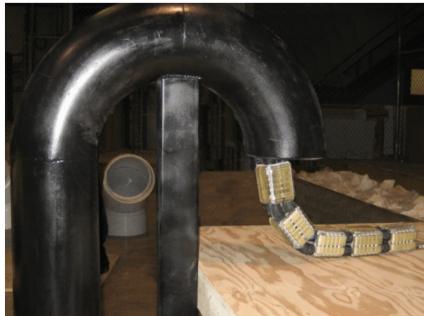
Fig. 1. The OmniTread Model OT-4 serpentine robot entering an "Inverted-'J'" ventilation duct at SwRI † .
