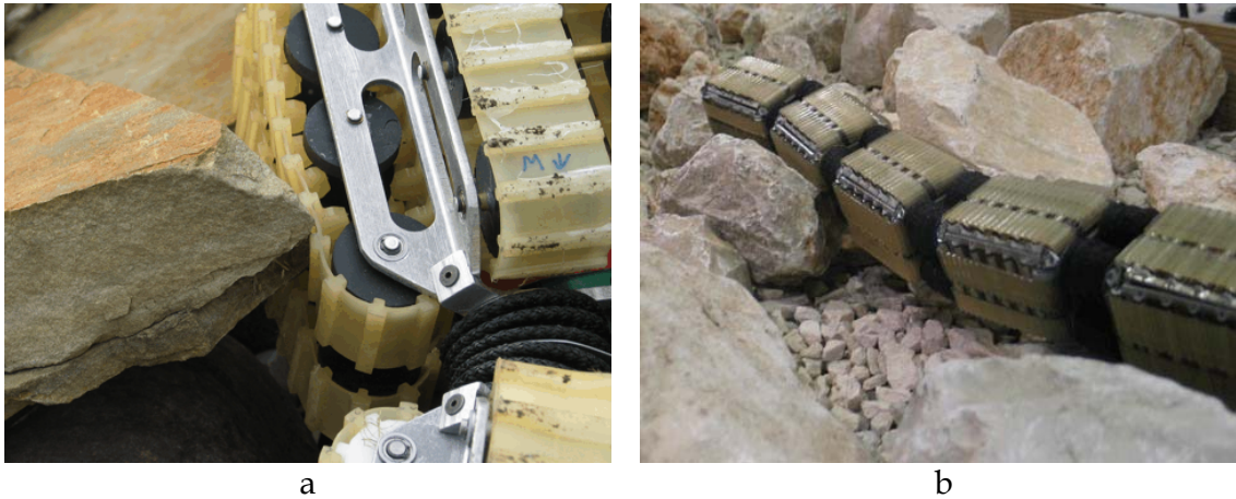
Fig. 5. Tracks all around: As the OmniTreads drive through rockbeds, it becomes apparent that side tracks help provide forward propulsion. a – OT-8; b – OT-4.
