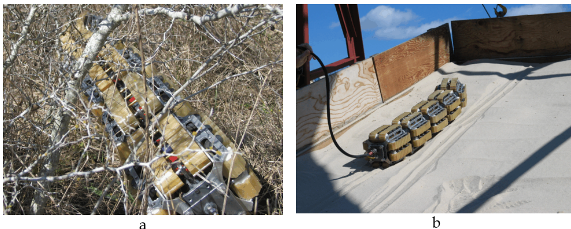
Fig. 11. The OT-8 outperformed the OT-4 on difficult natural terrains, mostly because of the OT-8 larger track sprocket diameter. a - The OT-8 literally plowed through SwRI's underbrush test area, aided, in part, by its more massive weight and greater power. b- Unaffected by sand, the OT-8 had enough power and traction to drive up a 15° inclined bed of deep sand.
