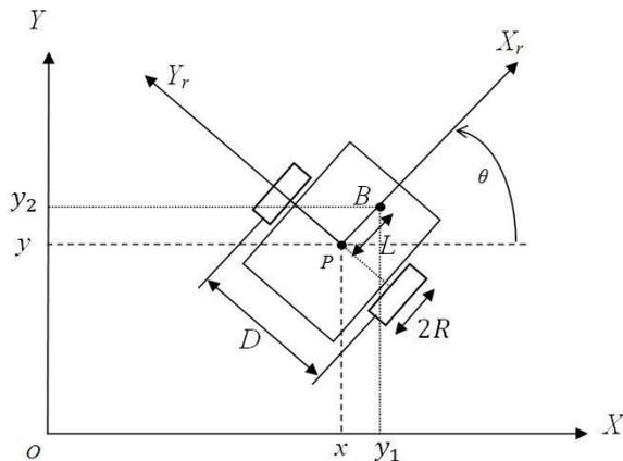
Figure 1: Unicycle mobile robot.
