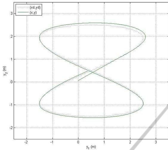
Figure 3: Asymptotic trajectory tracking using linear PID controller to track an eight shape trajectory on the  $(x,y)$  plane.
