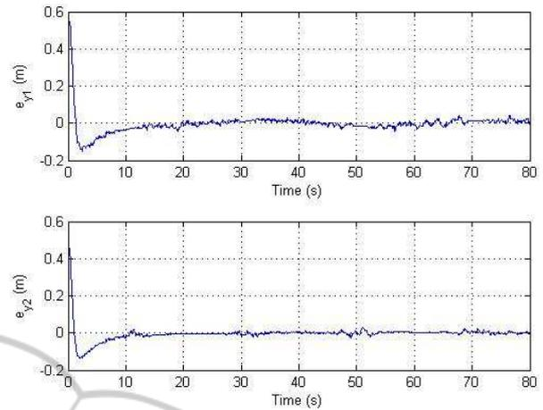
Figure 5: Output tracking errors using Integral Sliding Mode controller of an eight shape trajectory on the  $(x,y)$  plane.
