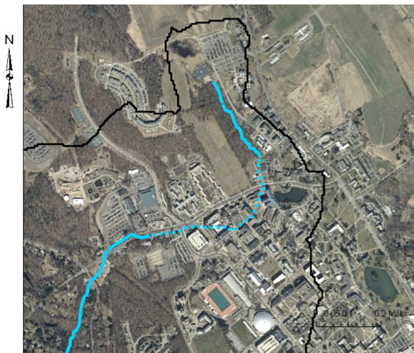
FIGURE 2: University of Connecticut campus in Storrs, with Eagleville Brook in blue (dashed blue line is where Eagleville Brook is in a concrete conduit beneath campus). Solid black line is watershed divide.
