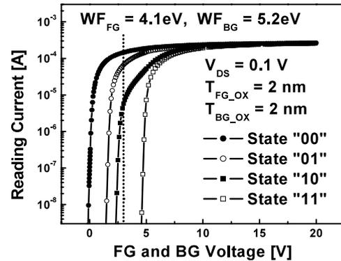
Fig. 6 I-V characteristics of the ASDG cell programmed with the 4 distinguishable states of “00,” “01,” “10,” and “11.”
