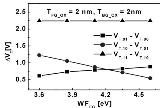
Fig. 7 A shift of threshold voltage for various front gate workfunctions.
