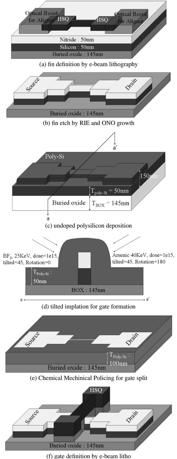
Fig. 2 Schematic diagrams of the process flow for a asymmetric Fin-FET SONOS device.
