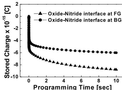
Fig. 4 The transient characteristics of the stored charge with V<sub>FG</sub> = V<sub>BG</sub> = 15 V on the nitride interface for states “11.”
