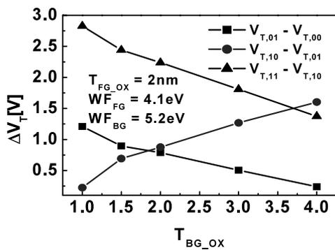
Fig. 10 A shift of threshold voltage for various back gate oxide thicknesses.
