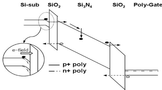
Fig. 5 The energy band diagram of the SONOS device during programming.
