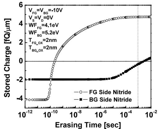
Fig. 12 Transient behaviors of the stored charges at the interfacial nitride of FG and BG side during the erase operation.
