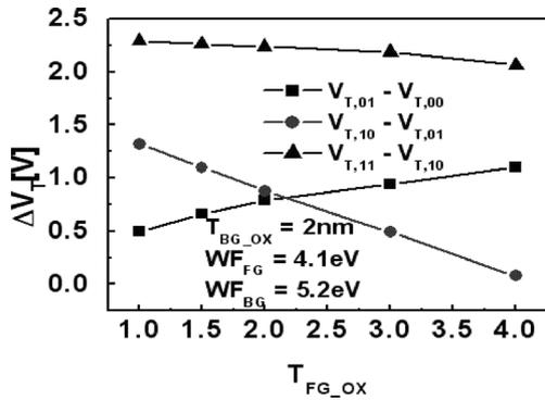
Fig. 9 A shift of threshold voltage for various front gate oxide thicknesses.
