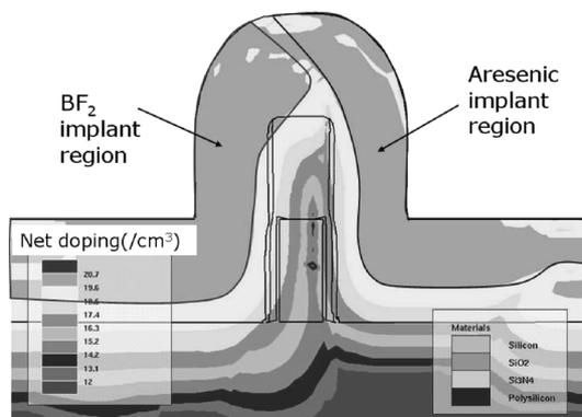
Fig. 3 Cross-section of ASDG FinFET along a-a' direction in Fig. 2(c) and shows the simulated doping profile after tilted implantation.
