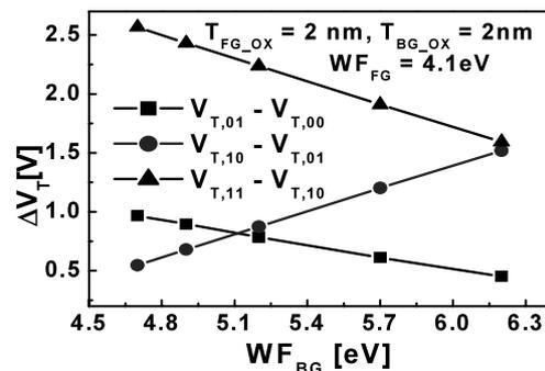
Fig. 8 A shift of threshold voltage for various back gate workfunctions.
