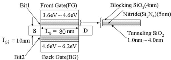
Fig. 1 Cross-sectional schematics of the ASDG NVM cell along a-a’ in Fig. 2(c).
