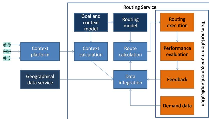
Figure 1: Key modules of the vehicle routing solutions.
